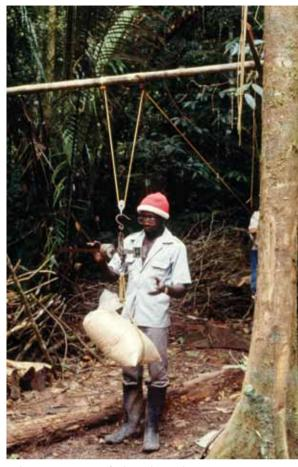
Photo 6.3. Measuring fresh weight saw dust, Mapane 1982. (Photo P. Schimdt)
